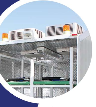
Aerodynamic roof design incorporated with LED warning lights (2 clear flashers & 2 red flashers & 2 oscillators) for greater visibility
